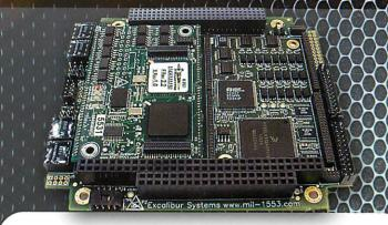
The **EXC-4000P104P** is designed for the PC/104-Plus standard for small, rugged, extended temperature boards. Designed to support our Dragon rugged avionics computer, it fits an amazing 5 modules in a very small area. These modules include 2 MIL-STD 1553 modules, one ARINC 429 module and two additional modules selectable from our full range of M4K modules.
