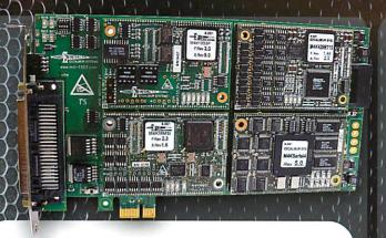
The **EXC-4000PCIe** is part of the 4000 family of multiprotocol carrier boards. This PCI Express interface board supports up to four independent and removable modules. Each module can be any of the 4000 family modules.
